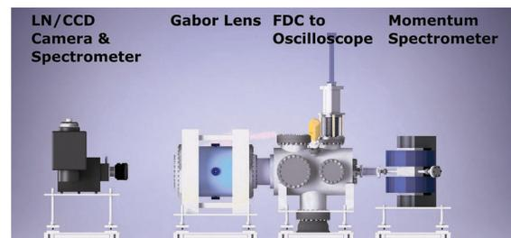
Figure 2: Experimental setup.
