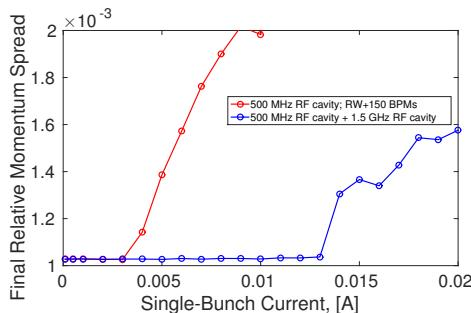
Figure 5: The single-bunch energy spread in the cases with and without the third harmonic cavity.
