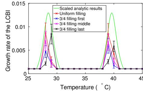
Figure 6: The comparison of the calculation of the longitudinal coupled-bunch instability driven by the longitudinal Higher-Order Mode L5 of the Cavity #3.
