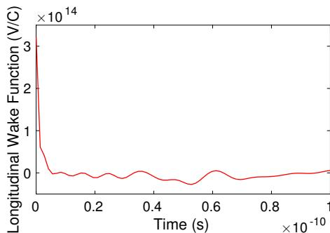
Figure 4: The total longitudinal wake function used in the simulations.
