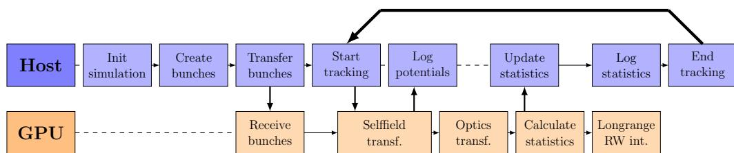
Figure 2: Flow diagram of mbtrack-cuda - tasks executed by CPU and GPU.
