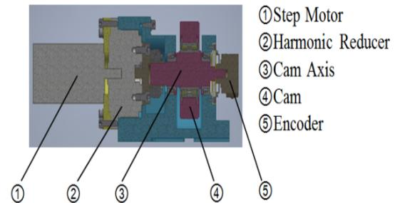
Figure 2: Mechanical design of cam motion system.
