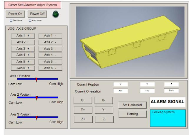
Figure 5: Test HMI.
