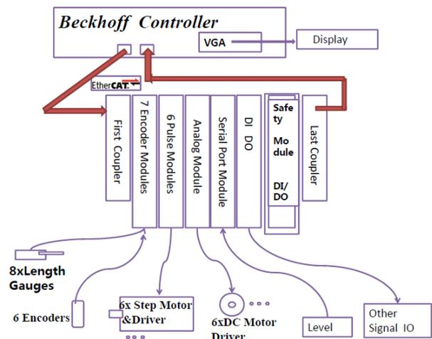
Figure 3: Control system frame.
