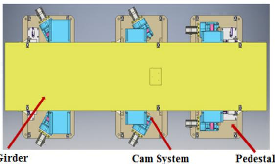
Figure 1: Structure of girder I.
