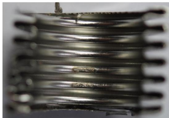
Figure 3: FPC push-rod bellow vacuum leak spot cut-out.
