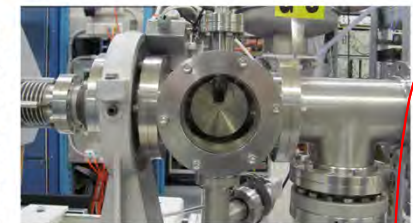
Figure 1: The target station of the beam pulse profile monitor. The target, as seen through the viewing port, can be moved in/out and is rotated by 45 degrees with respect to the beam.
