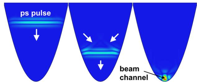
Figure 2: E-field distributions at the parabolic mirror while focusing the short THz pulse, for the time correspondent to beginning of focusing at  $t=3.6$  ps (left), for time when focusing is close to maximum at  $t=7.6$  ps (center), and in maximum of focusing (right) at  $t=11.6$  ps.
