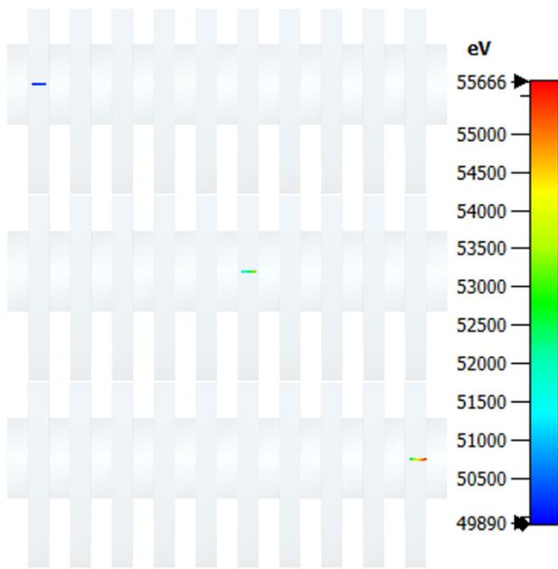
Figure 5: Bunch acceleration for three sequent time frames: top – bunch enters the first cell ( $t=11.6$  ps), center – bunch crosses middle line ( $t=15.6$  ps), bottom – bunch arrives the end ( $t=18.8$  ps).
