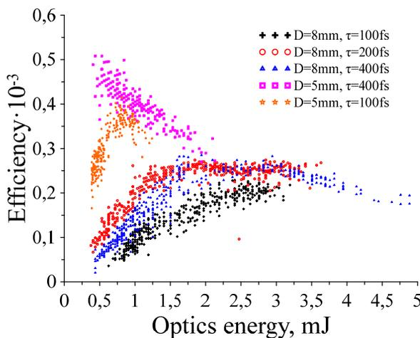
Figure 6: Efficiency of optical to THz radiation conversion in  $\text{LiNbO}_3$  vs optical pulse energy for different pulse lengths and laser beam sizes.
