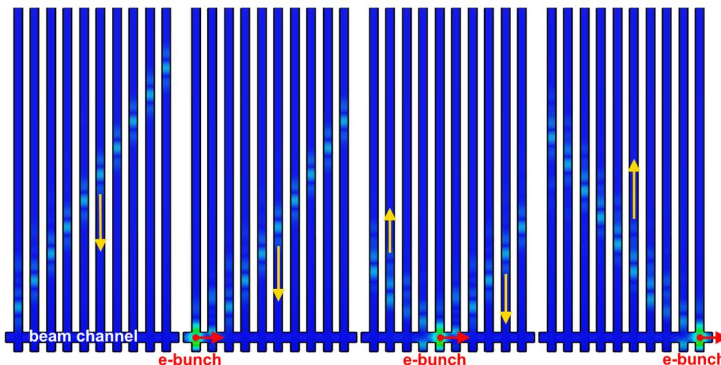
Figure 4: Front view of dielectric delay line THz accelerating structure (time proceeds from left to right).
