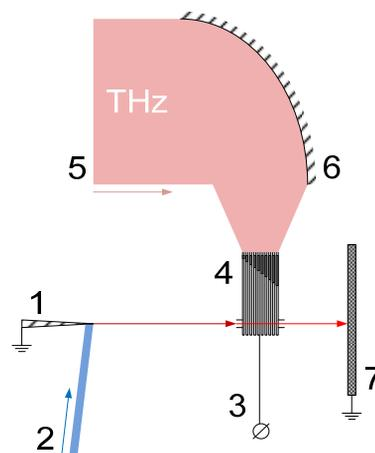
Figure 10: Sketch of experimental setup based on deceleration section measurements: 1 – needle cathode, 2 – laser beam, 3 – accelerating section, 4 – THz accelerating structure, 5 – THz beam, 6 – parabolic focusing mirror, 7 – deceleration section, 8 – YAG screen.
