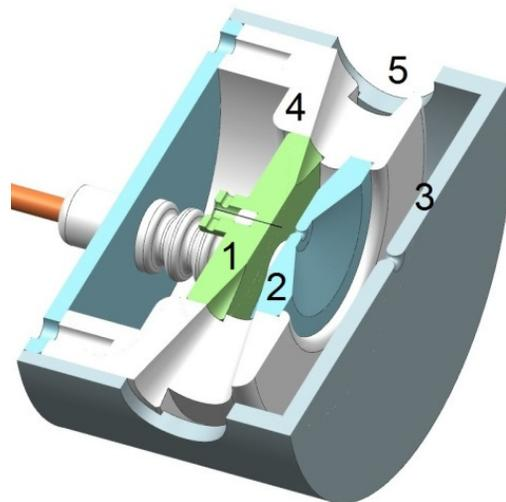
Figure 8: Electron DC acceleration gun: 1 – needle cathode, 2 – intermediate anode, 3 – main anode, 4 – insulator, 5 – gate for laser beam.
