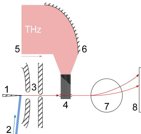
Figure 9: Sketch of experimental setup based on spectrometer measurements: 1 – needle cathode, 2 – laser beam, 3 – accelerating DC gun, 4 – THz accelerating structure, 5 – THz beam, 6 – parabolic focusing mirror, 7 – spectrometer, 8 – YAG screen.
