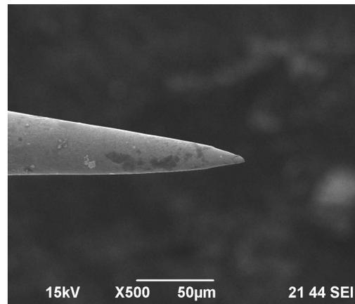
Figure 7: Tungsten cathode needle as shown in electronic microscope.
