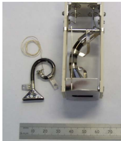
Figure 1: Channeltron on left is the 4800 series of the Channeltron array. On the right is the 4700 series still used in the old SCPM.
