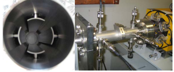
Figure 1: Picture of the stripline transverse geometry (left), and stripline as installed in the ALBA Booster. The electrode covering angle is 60^\circ .
