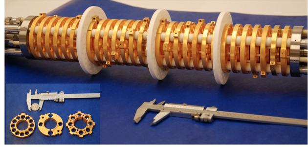
Figure 2: CPET assembly and its electrodes on the inset. A Canadian 25 cent coin is shown with the slide callipers.
