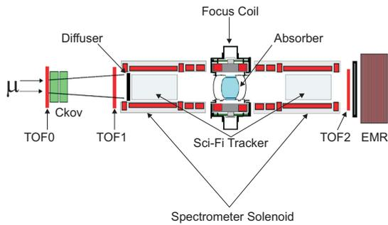
Figure 4: Schematic of MICE Step IV with the two spectrometer solenoids, diffuser, absorber and focus coil.
