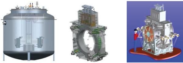
Figure 4: (a) FNAL test configuration for coupling coils, (b) final RFCC cryostat and (c) the RF module and coil.
