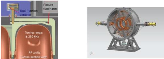
Figure 5: Cavity section showing tuning arm system, and view of the single cavity test stand at the MTA.
