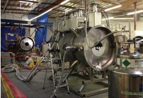
Figure 3: The first spectrometer solenoid training (foreground) whilst the second completes assembly.
