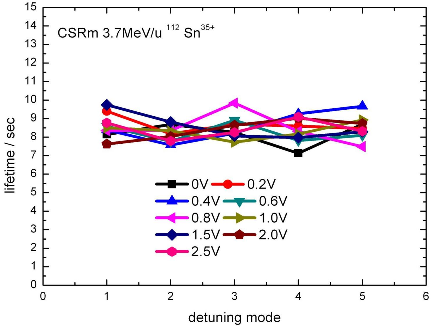
The voltage amplitude of modulation was not sensitive to the lifetime of ion beam.
