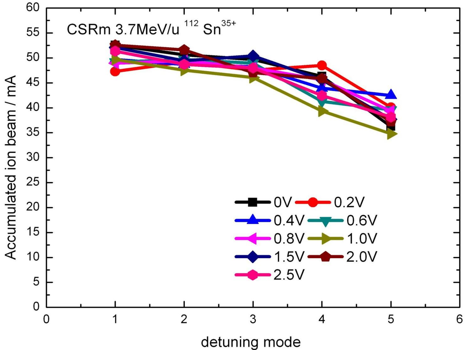
Due to the ion beam intensity gradually became smaller from the injection during the experiments, the accumulated ion intensity became smaller too.
