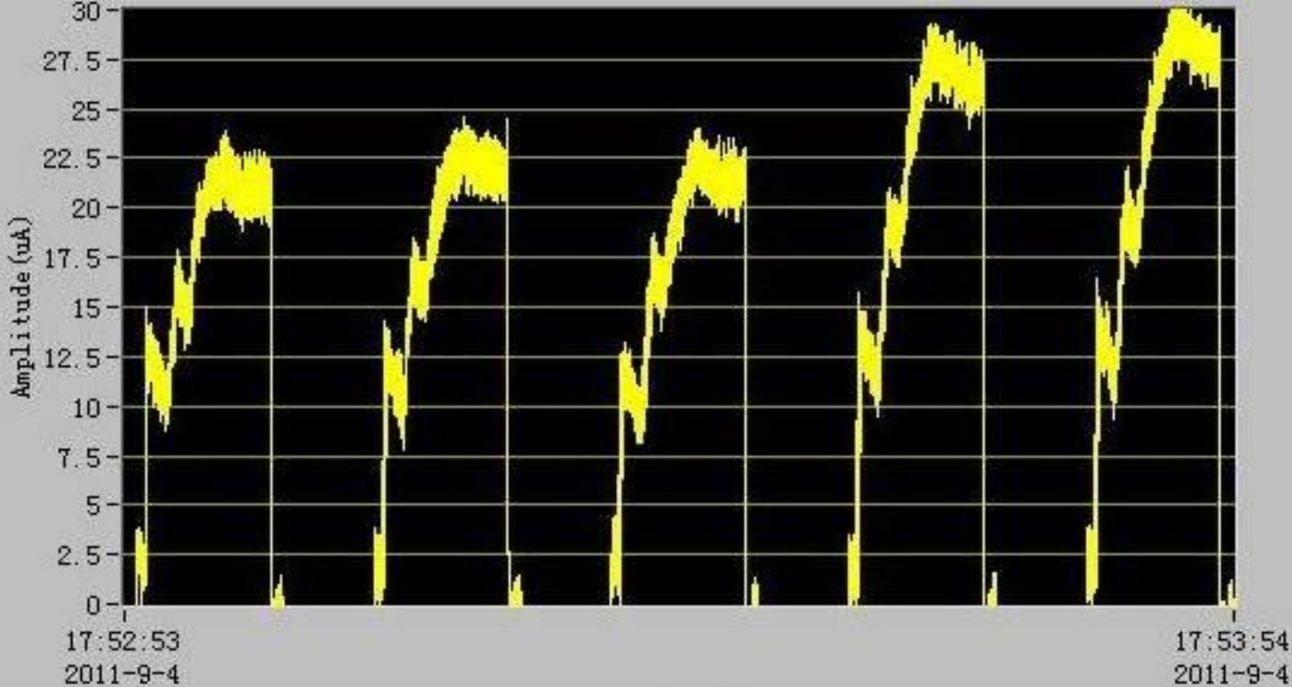
The proton beam disappeared after turn on the electron cooler and electron beam. There was no obvious cooling and accumulation. The lifetime of  $H^+_2$  is very short comparing with the results from TSR and CELSIUS.
