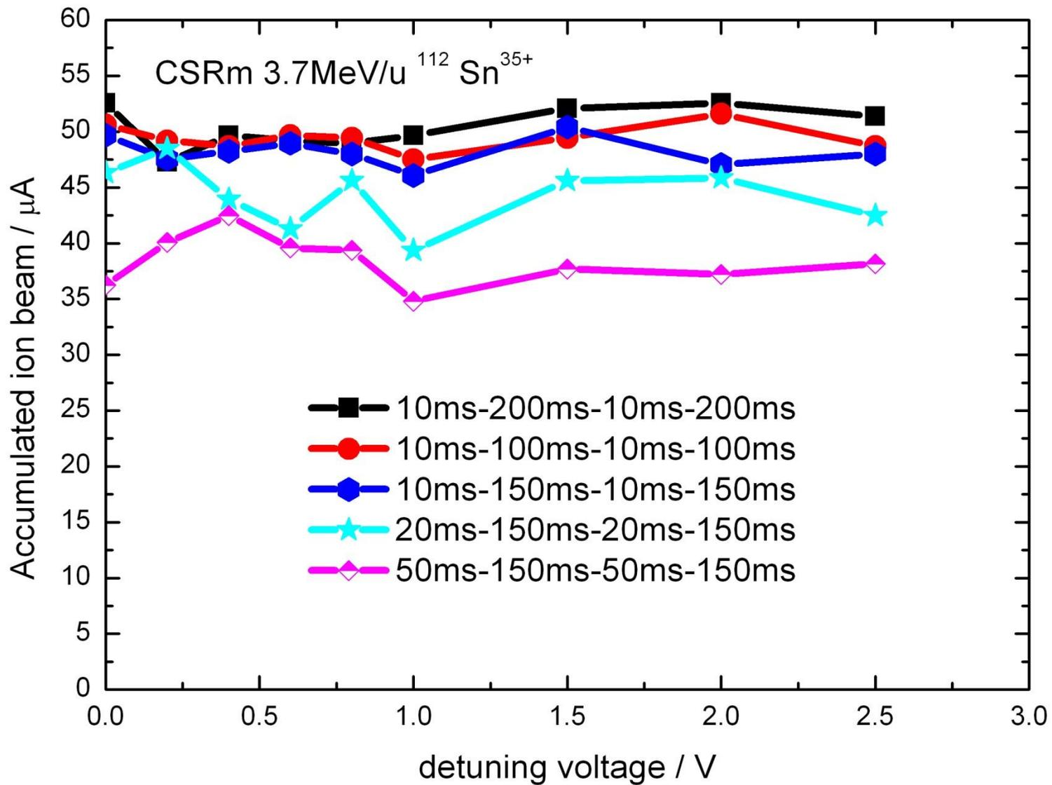
The voltage amplitude of modulation was not sensitive to the accumulated ion intensity.
