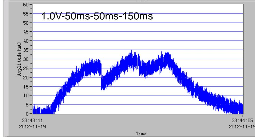
The DCCT signals with the modulation interval
