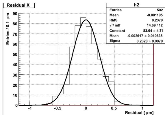
Figure 1: Position correlation between three SCSS cavity BPMs, corresponding to less than 200 nm resolution [12].
