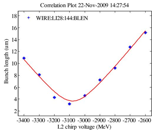
Figure 2: Scan of the LCLS rms bunch length after the second bunch compressor vs. chirp voltage in the L2 linac [22].
