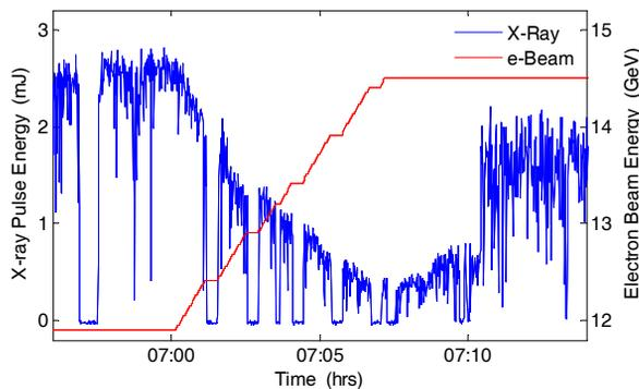
Figure 4: LCLS X-ray pulse energy during energy ramp from about 12 to 14.5 GeV. The jump in photon energy around 7:10 is due the recalibration of the gas detector [36].
