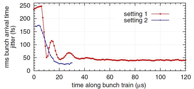
Figure 3: Beam arrival time jitter reduction to 20 fs with intra-bunch feedback at FLASH [30].
