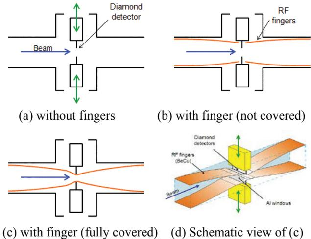
Figure 1: Configuration of the RF fingers.
