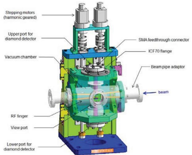
Figure 4: The mechanical design of the halo monitor.
