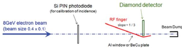
Figure 2: Setup of experiment at synchrotron beam dump.
