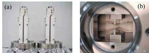
Figure 5: Photograph of (a) detectors with microstripline structure, and (b) RF fingers with Al windows (beam direction: from left to right).
