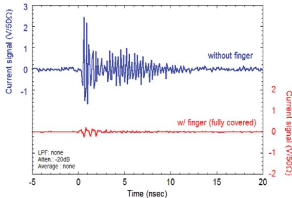
Figure 6: The suppression of effect of wake field.
