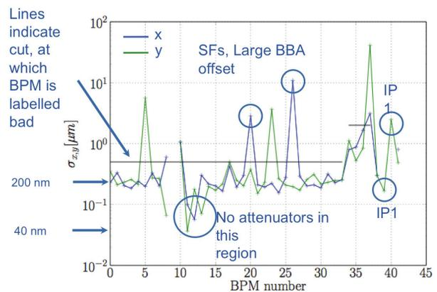
Figure 3: CBPM residuals measured along the ATF2 extraction beamline.
