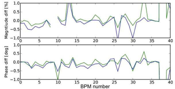
Figure 2: Fluctuations of the amplitude and phase calculated using calibration tone data covering 4 days.
