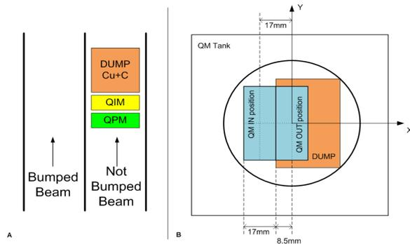
Figure 2A: Top view of the QM position – 2B: IN and OUT Qualification Monitor position with respect to the tank and the dump.
