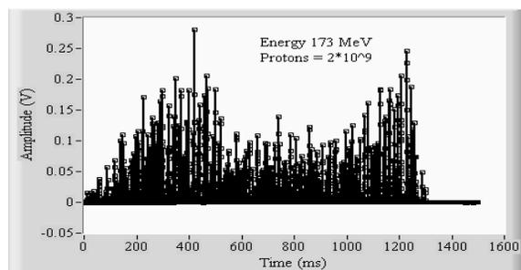
Figure 5: Beam intensity versus time. The amplifier gain is G5 and the acquisition rate is 10 kHz.
