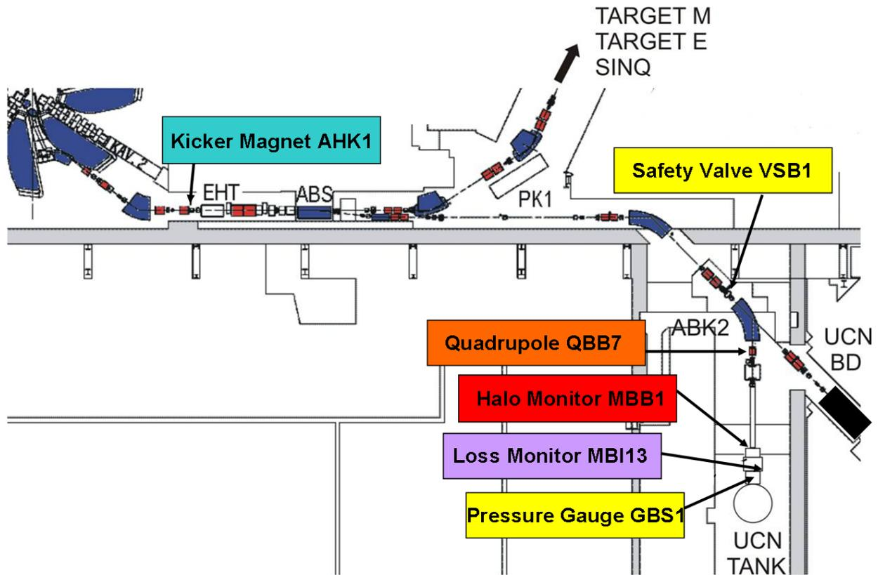
Figure 1: A schematic view of the UCN beam line. The 590 MeV, 1.3 MW proton beam delivered by the ring cyclotron is diverted to the UCN beam line by means of the fast kicker magnet AHK1 followed by the septum magnet ABS with a duty cycle of 1 %. The elements belonging to the UCN-SAS beam safety system are displayed in the coloured boxes.
