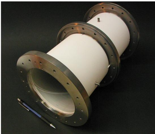
Figure 2: Photo of a ceramic BPM. Metal-deposited areas on inner surface serve as signal pick-ups.
