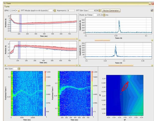
Figure 3: TOPOS GUI for tune measurements: Top and centre: x and y position vs. time at a selected BPM in min/max representation (left) and online FFT of position data (right). Bottom: hor. and vert. tune vs. time and working diagram of SIS18 with online tune values (red).
