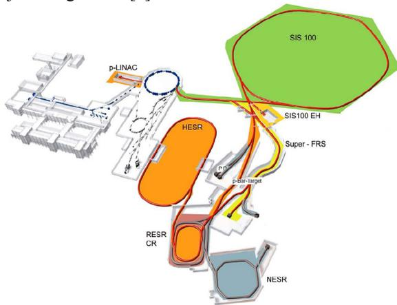
Figure 1: Existing GSI and layout of the FAIR accelerator complex (NESR and RESR not part of the start version).
