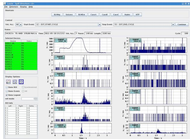
Figure 4: LASSIE GUI showing current transformer data (top left) and 11 beam-loss monitors along SIS18.
