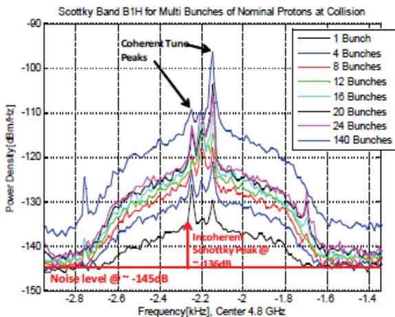
Figure 5: Incoherent Schottky Bands for protons at Collision.
