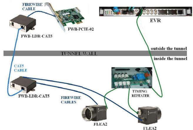
Figure 4: FireWire camera cabling, blue: signal cables, green: timing cables. Details in the text.
