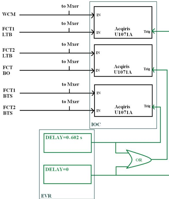
Figure 2: Schematics of the Acqiris cards cabling. All abbreviations are detailed in the text, except Mxer: Multiplexer.
