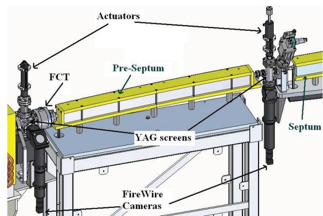
Figure 1: Drawing of the end of the BTS showing the location of the new FCT and the two new YAG:Ce screens, on both sides of the SR injection pre-septum.
