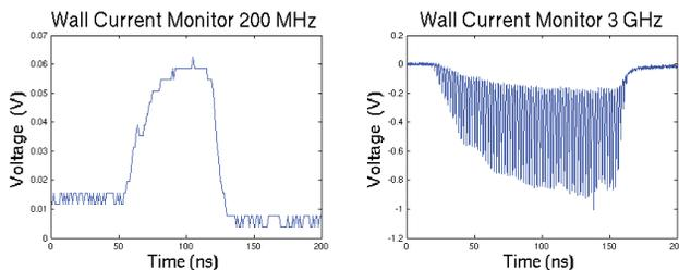
Figure 3: WCM signal observed at 3 GHz (right) with an oscilloscope and 200 MHz (left) with the Acqiris card [6].
