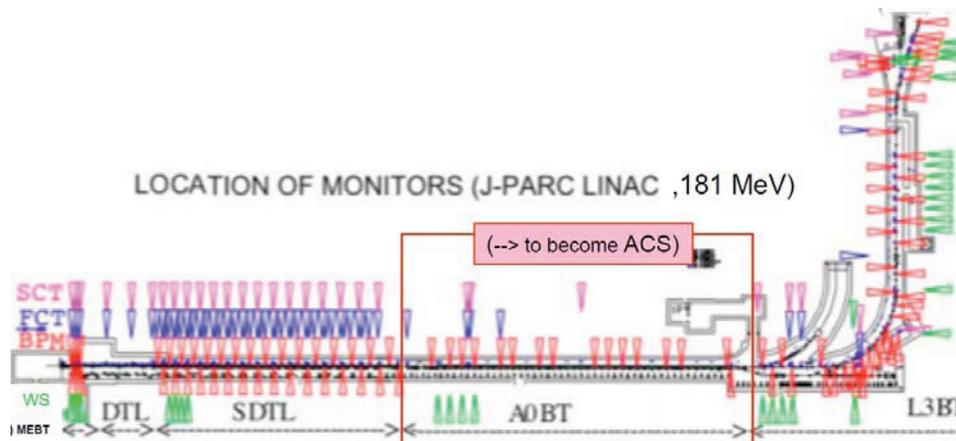
Figure 1: Location of beam monitors in present J-PARC linac. Pink marks are SCT monitors, blue are FCT monitors, red are BPM monitors and green are profile monitors respectively. Beam transport (A0BT) in the red square will become the ACS section where the ACS cavities will be installed.
