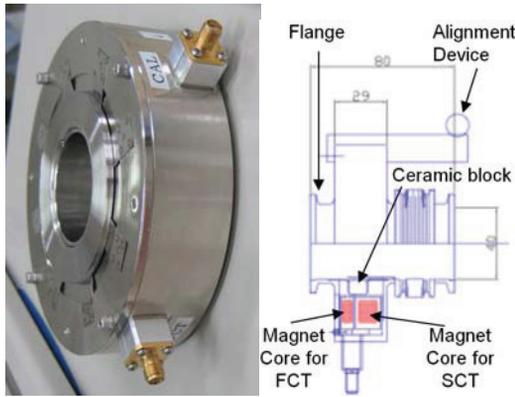
Figure 2: Beam current and phase monitor (SCT/FCT).
