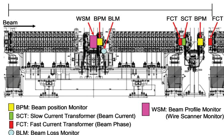
Figure 3: Typical layout of the beam diagnostic devices between the ACS cavities.
