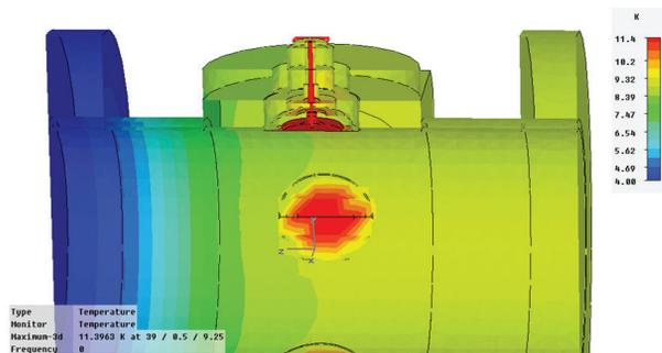
Figure 3: Temperature simulation [4] result of a copper button with highest power at the European XFEL.
