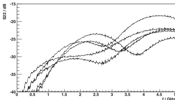
Figure 8: Measured reflection as a function of frequency of the warm button with adapter.
