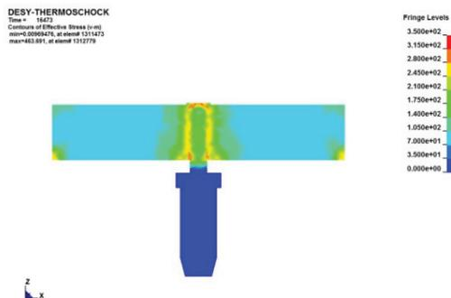
Figure 6: The stress of the inner pin at the vacuum barrier of the feedthrough.
