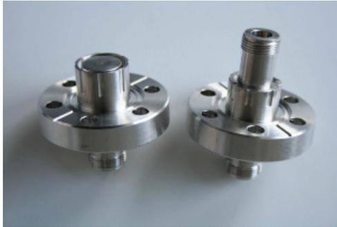
Figure 7: Photo of the warm button, with button (left) and with adapter (right).
