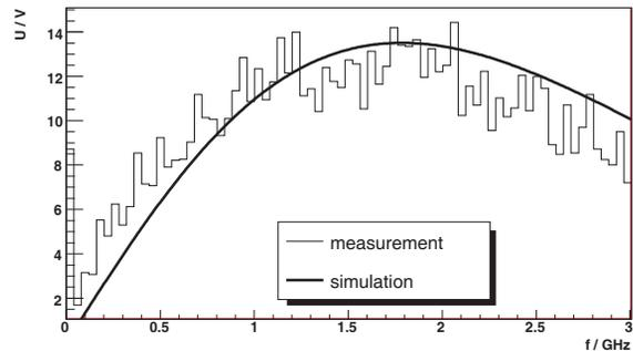
Figure 9: Measurement of the electrical spectrum from the warm button at 0.9 nC compared with a scaled simulation result [4].
