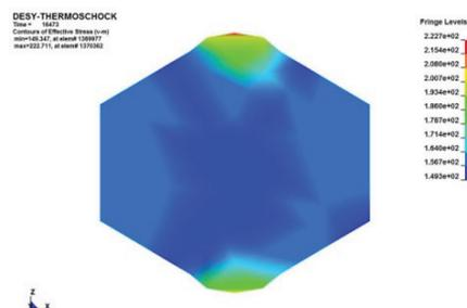
Figure 5: The deformation of the gasket cross section is shown. The contact is on top and bottom.
