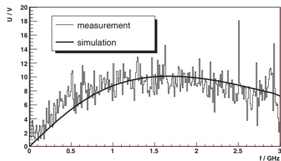
Figure 2: Measurement of the electrical spectrum from the button compared with a scaled simulation result [4].
