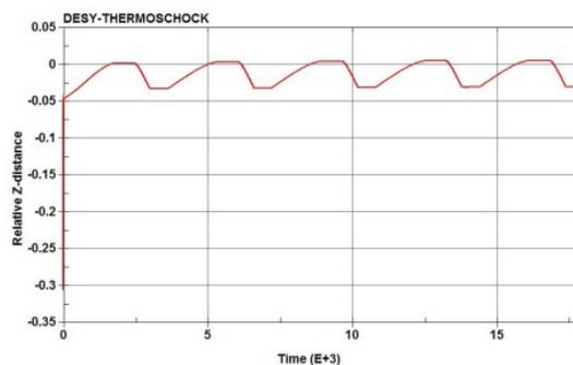
Figure 4: Position of the button in mm as a function of time. The thermo cycles are visible.
