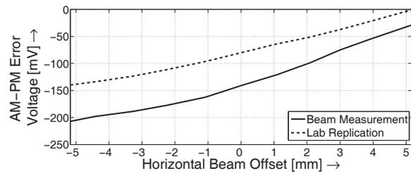
Figure 3: Solid: DC error voltage generated by AM-PM-processing of an S-Band beam moved horizontally between capacitive pickups. Dashed: Lab measurements using the same receiver but RF generators emulating the test stand's beam signals (RF power is -7 dBm at the mixer input).
