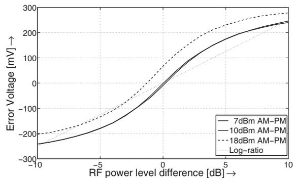
Figure 7: Measurement results of AM-PM-generated error signal for different power levels compared to an exemplary  $V_{DC} - P_{RF}$ -curve generated by log-ratio processing.
