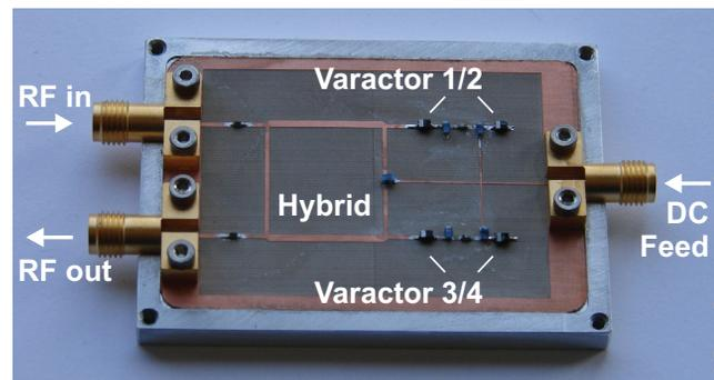
Figure 4: Planar phase shifter employing four varactor diodes Infineon BB 837 (0,55...6,6 pF over 0...25 V).
