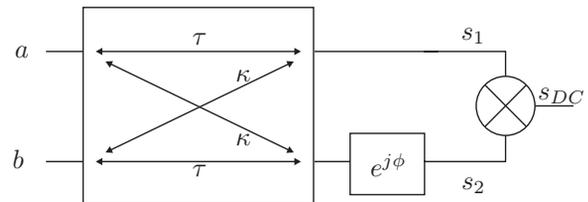
Figure 1: Sketch of an AM-PM frontend comprising one hybrid, delay line and mixer per measurement plane.
