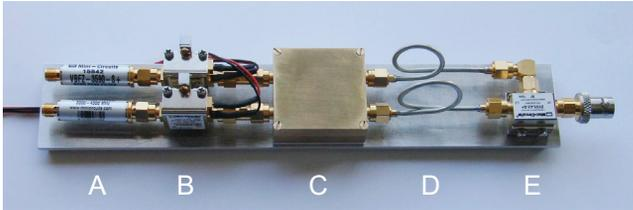
Figure 2: Discrete implementation of AM-PM prototype.
