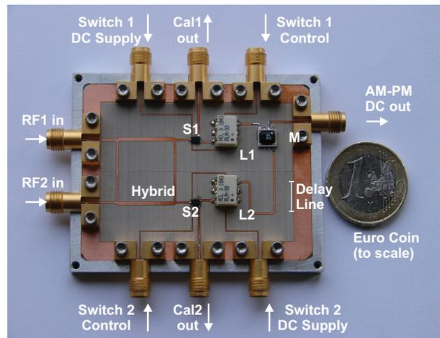
Figure 6: Planarized AM-PM receiver module fabricated on Arlon CLTE-AT substrate (S1/S2: Switches, L1/L2: Limiters, M: Mixer).
