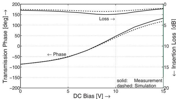
Figure 5: Adjustable phase range and insertion loss of planar varactor-based phase shifter.
