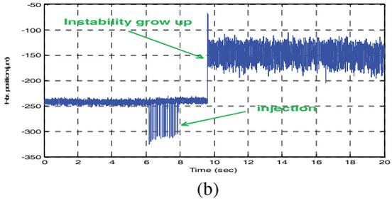
Figure 5: (a) The four blades reading for transverse bunch-by-bunch feedback on/off (b) the horizontal photon beam position change for TBF on/off
