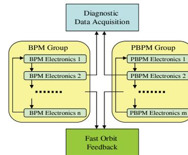
Figure 1: Fast links of electrical and photon BPM
