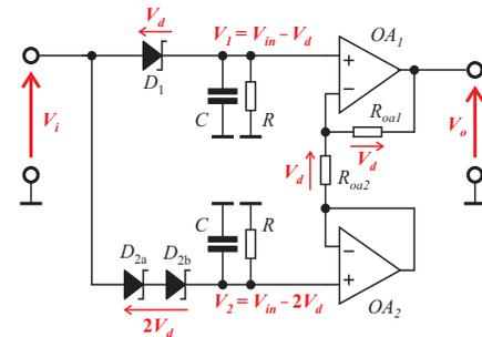
Figure 1: Compensated diode peak detector diagram.
