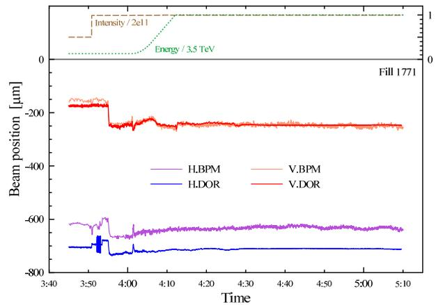
Figure 3: Beam orbits from the BPM and DOR systems.
