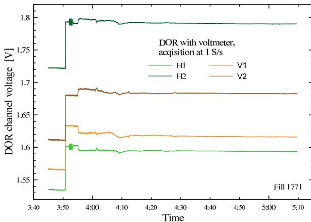
Figure 2: Raw signals from the DOR system.
