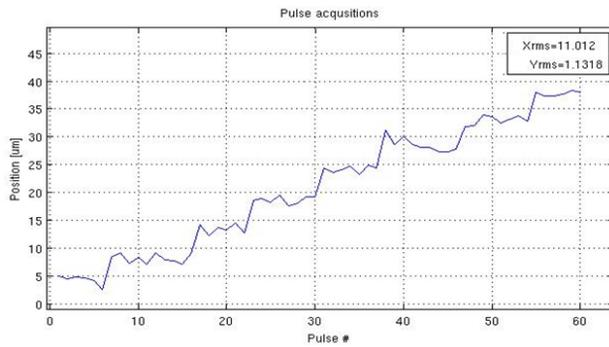
Figure 5: Wire movement – by 5 um steps in X-direction. Seven steps are seen in position measurement.
