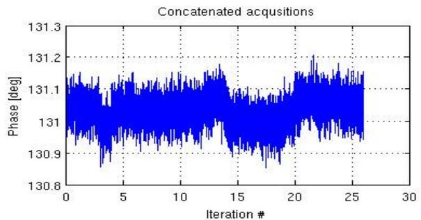
Figure 4: Negligible impact of the off-centered beam on the phase measurement.
