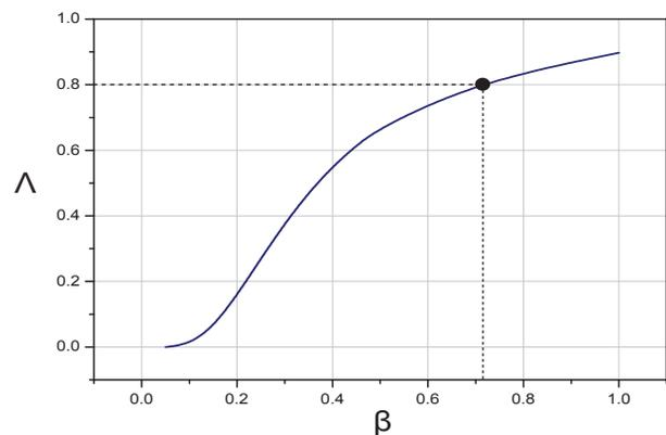
Figure 4: Transit Time Factor  $\Lambda$  as a function of beam velocity  $\beta$
