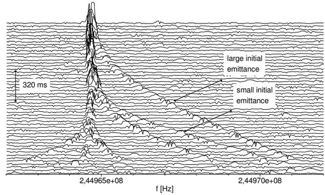
Figure 5: Waterfall diagram showing electron cooling of six  $^{142}\text{Pm}^{59+}$  ions
