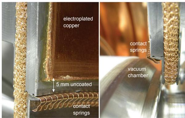
Figure 2: Detailed views of a corner of one half-shell. The left picture shows a view on the electroplated copper surface with the uncoated region and the rf contact springs, the right picture shows how a half-shell can be mounted on the vacuum chamber. In both pictures, rf currents propagate vertically on the half-shell in the fundamental mode.
