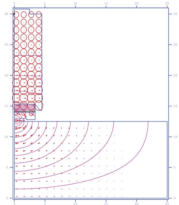
Figure 3: Simulated field pattern in one quarter of the resonator. The lines represent electric field lines, whereas circles illustrate the magnetic field strength.
