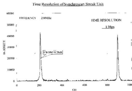
Figure 8: Time resolution of the Streak unit.
