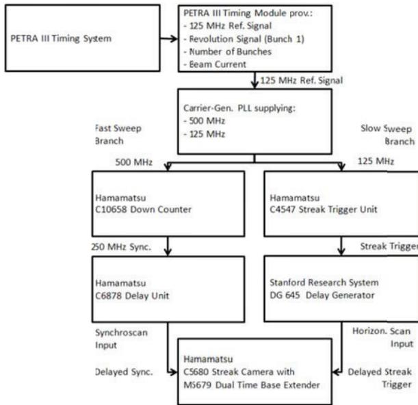
Figure 7: RF system signals for the Streak camera.
