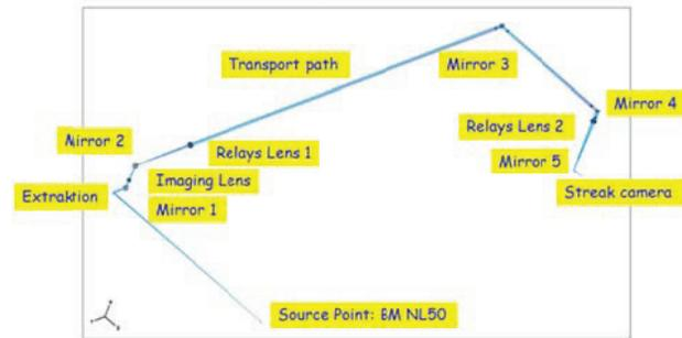
Figure 5: Optical path from magnet to Streak camera.
