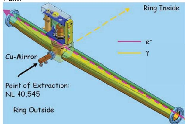
Figure 2: Light extraction vessel.
