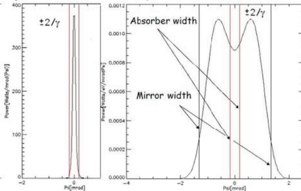
Figure 3: Left: Total radiation power over  $\phi=2,8 \text{ mrad}$ , right: same at 2 eV.
