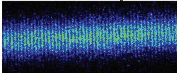
Figure 10: Part of bunch train of 50 mA with 72 bunches.
