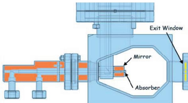
Figure 4: Copper mirror, absorber and exit window.
