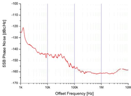
Figure 3: SSB Phase Noise measured at 1326 MHz (17<sup>th</sup> Harmonic of fundamental signal).
