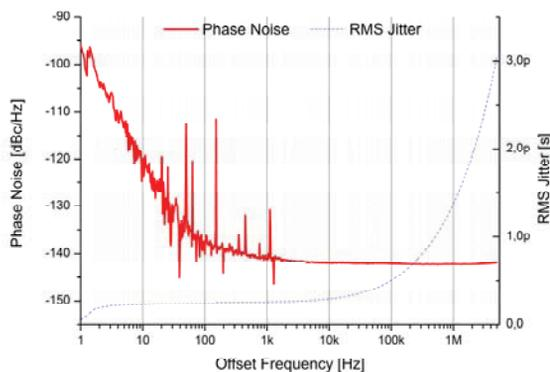
Figure 1: Phase Noise (solid line) and RMS-Jitter (dashed line) of 13 MHz after cw distribution.
