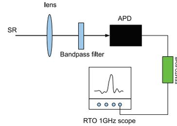
Figure 1: Experimental setup. The filtered synchrotron radiation is focussed onto Perkin Elmer C30302S-DTC APD. Then the APD signal is amplified by a FEMTO 60 dB amplifier before being recorded by Rohde & Schwarz RTO scope.
