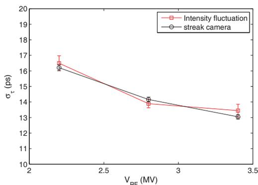
Figure 3: Bunch length as function of the RF cavity voltage, measured with the intensity fluctuation using a  $632 \pm 5 \text{ nm}$  filter (FWHM bandwidth).
