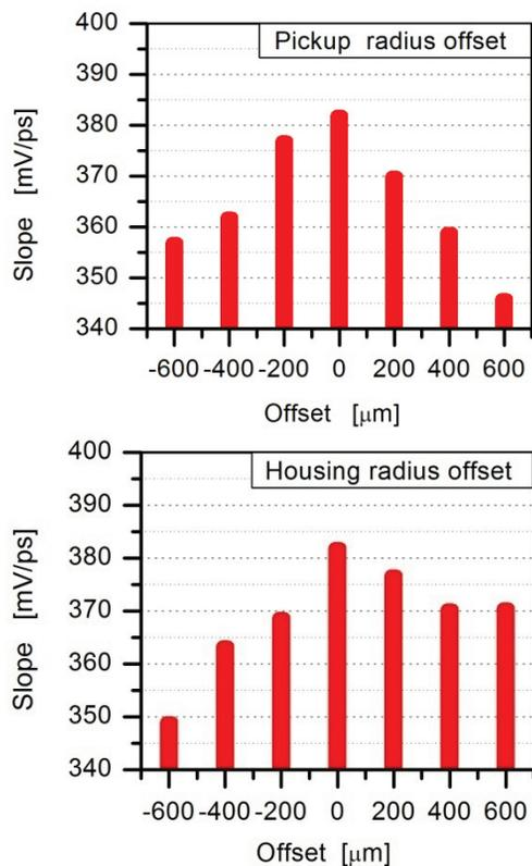
Figure 5: Top: pickup radius, Bottom: housing radius.
