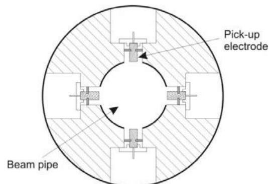
Figure 2: Cross-section of a button type beam pick-up for a BAM.
