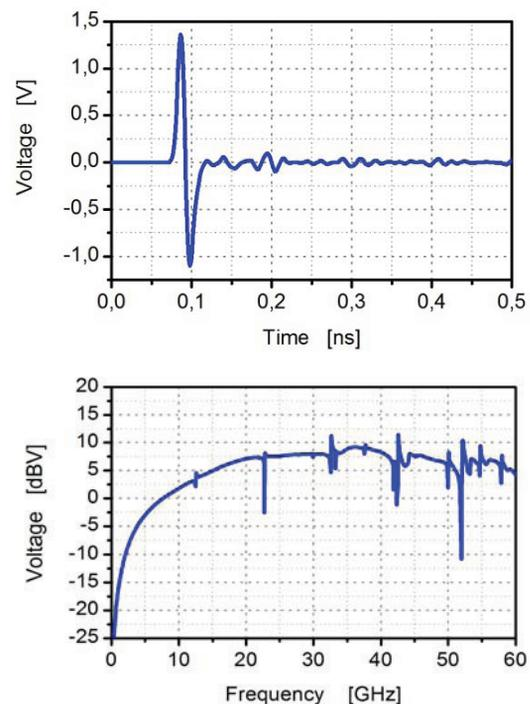
Figure 4: Beam pickup signal: Top: time domain, Bottom: frequency domain.
