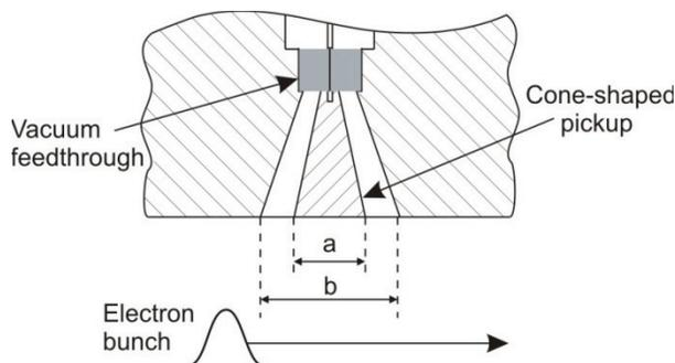
Figure 3: Cross-section of the cone-shaped pickup electrode for the BAM.
