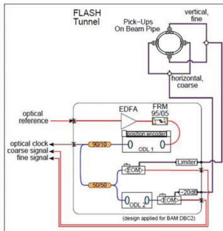
Figure 1: BAM electro-optical front-end.
