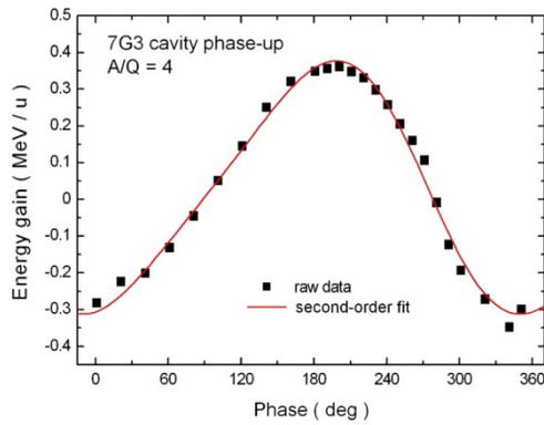
Figure 4: Demonstration of cavity phasing with the REX 7-gap resonator.
