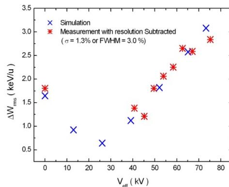
Figure 3: Simulated and measured energy spread as a function of the rebuncher voltage.
