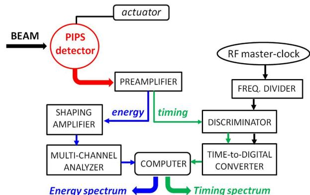
Figure 1: Monitor structure and data acquisition setup.
