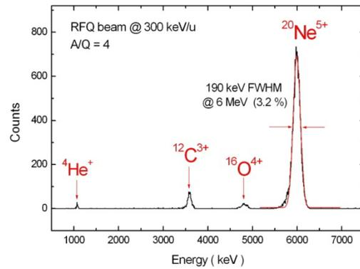
Figure 2: Beam energy spectrum acquired at 300 keV/u.
