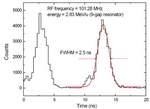
Figure 5: Beam timing profile and bunch length.
