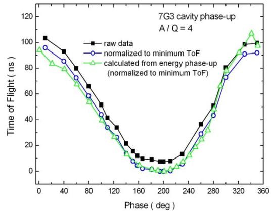
Figure 6: Phase scanning of the 7G3 cavity through ToF measurements.
