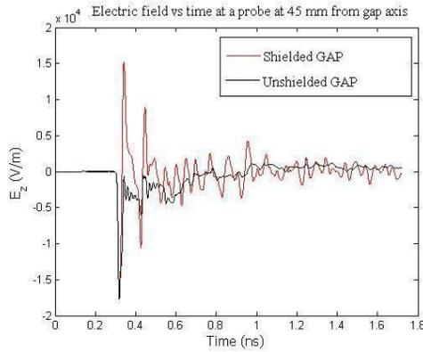
Figure 7: Comparison, in time domain, between the field radiated by the shielded and unshielded structures.
