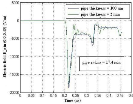
Figure 2: Temporal trend of the z-component of the electric field in the point (0.45,0.0,0.0), in which there is the probe.
