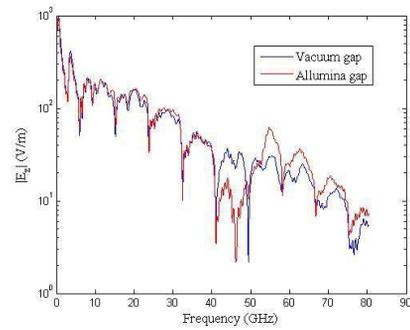
Figure 4: Comparison between vacuum gap and alumina filled gap model, in frequency domain.
