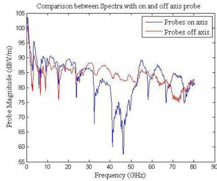
Figure 5: Comparison between field radiated in case of probe on x-axis.
