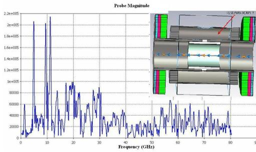
Figure 6: Complete gap model, and frequency domain simulation result.
