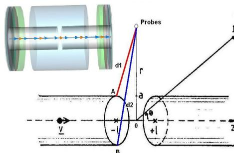
Figure 1: Model of the gap used in CST for the simulation of the energy radiated by the gap (left top) and scheme of the analytic model from [5]
