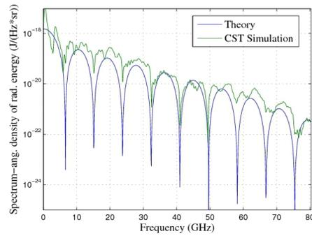
Figure 8: Comparison between simulation results and theoretical formulation of the spectrum-angular energy radiated by the gap.
