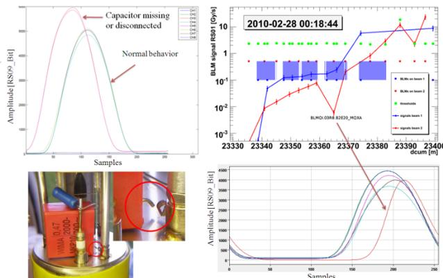
Figure 3: Modulated signal (left-top) with a non-conformity on the HV input filter (left-bottom). Detector sensitivity loss due to non-conformity of the tunnel card discovered with beam (right-top) and confirmed by the connectivity check (right-bottom).
