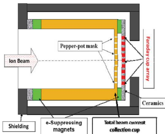
Figure 2: Schematic diagram of the pepper-pot beam profile measurement device.
