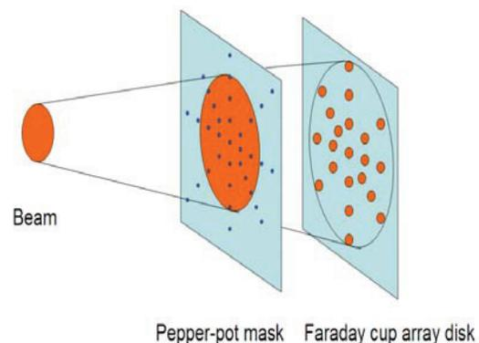
Figure 1: The beam profile measurement principle.
