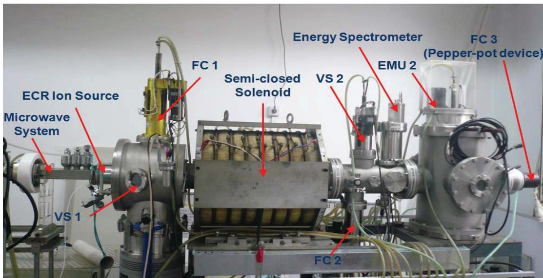
Figure 4: Low Energy Beam Transport (LEBT) Test Bench.
