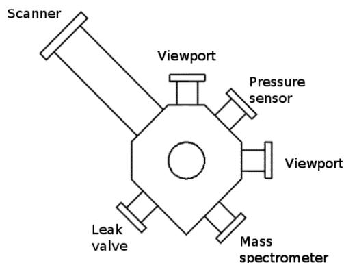
Figure 2: Vacuum chamber for beam induced fluorescence studies. The electron beam goes into the plane of the paper
