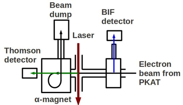
Figure 4: Schematic view of the future diagnostic setup at the PKAT
