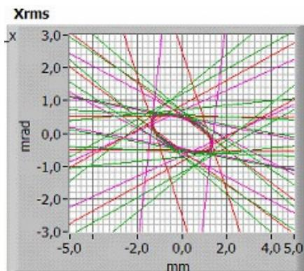
Figure 6: Emittances picture from BCSM (green lines) and wire scanners (red lines).
