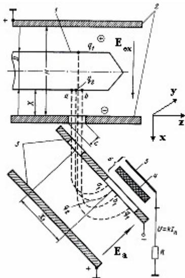
Figure 2: BCSM scheme: 1-Particle beam, 2-Ion extractor with slit, 3-Electrostatic analyzer, 4-MCP image intensifier, 5-Luminescent screen, 6-Electro-Optical Converter.
