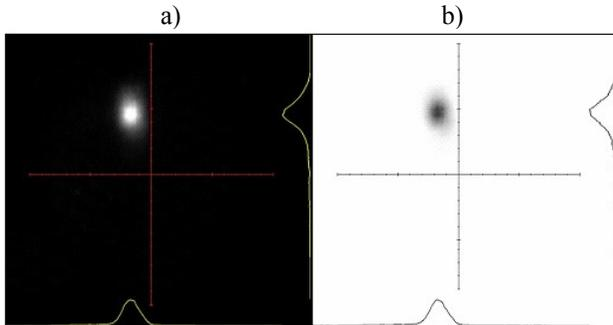
Figure 5: On-line images of INR proton beam cross section: a) 1 Hz, 200  $\mu$ s, 14 mA pulse current, b) 1 Hz, 3  $\mu$ s, 10 mA pulse current.
