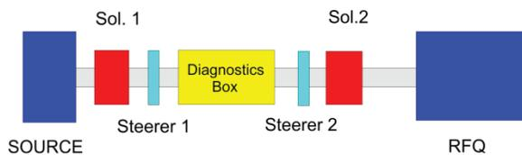
Figure 1 Diagram of the LINAC4 LEBT.
