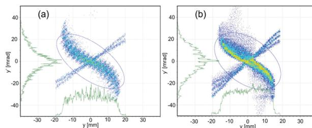
Figure 4: Simulated (b) and measured (a) phase space after the first solenoid, for  $I_{sol1}=600$  A.
