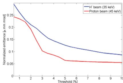
Figure 2: Normalized emittance measured for a proton beam at 45 keV and H<sup>-</sup> beam at 35 keV as a function of the threshold applied to the data.
