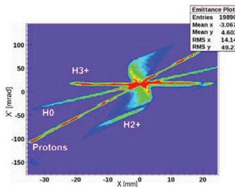
Figure 3: Different particle types separated by solenoid.
