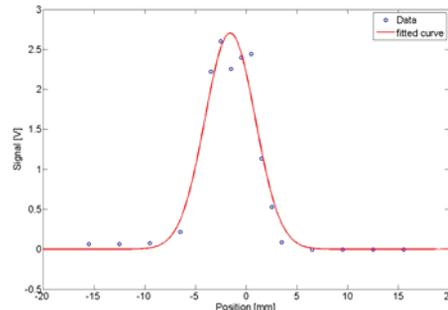
Figure 5: Reconstructed profile and Gaussian fit at the end of the spectrometer line.
