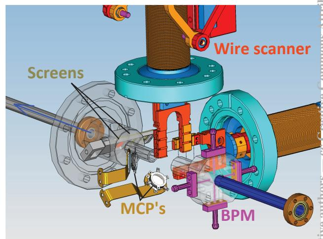
Figure 1: The diagnostic unit to measure the transverse properties of the electron and the photon beam consists of a beam position monitor (BPM), a vertical and a horizontal wire scanner, an aluminum coated silicon screen and a cerium-doped YAG screen [4]. Two micro-channel plates (MCP) close to the wires are used to measure photoelectrons emitted from the wire after the XUV laser interacts with it. The blue arrow indicates the beam direction.
