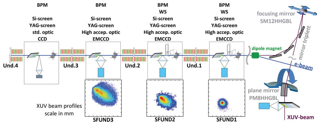
Figure 2: The schematic of the sFLASH beamline, it illustrates the injection beamline for the seed laser and the beam diagnostic stations. Exemplary XUV beam profiles along the undulator using a mirror with a focal length of 6.25 m.
