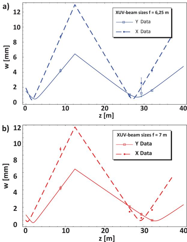
Figure 4: Results of beam size measurements of the XUV beam along the sFLASH injection beamline for different focal length. The dashed and solid lines are fits to the data points using a Gaussian beam transport model. With that, the XUV beam parameter in the undulator can be estimated.
