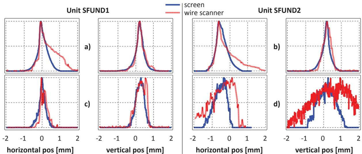
Figure 3: Electron beam profiles (upper row a) and b)) and XUV laser beam profiles (lower row c) and d)) each measured with cerium-doped YAG screens and EMCCD cameras (blue lines) and with wire scanners (red lines) after adjusting the transverse laser position. The profile intensity is normalized for each measurement.
