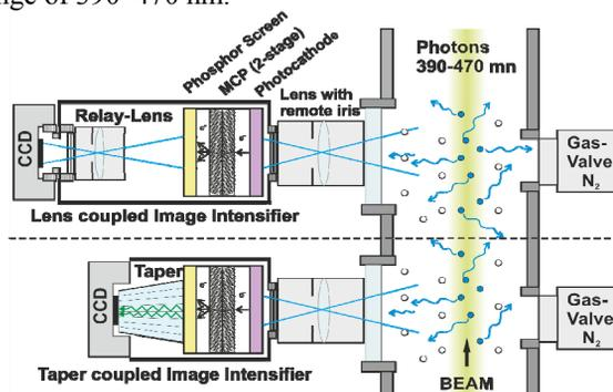
Figure 1: BIF detection principle with relay coupled (top) and taper coupled (bottom) CCD camera.
