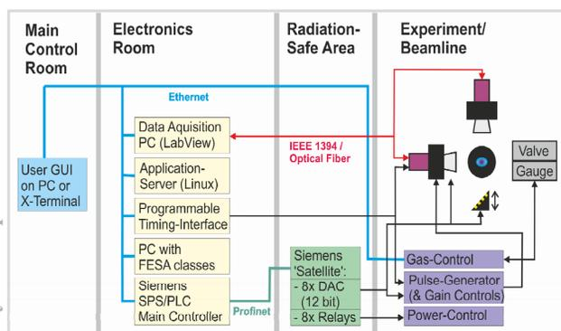
Figure 3: BIF electronic devices and communication.
