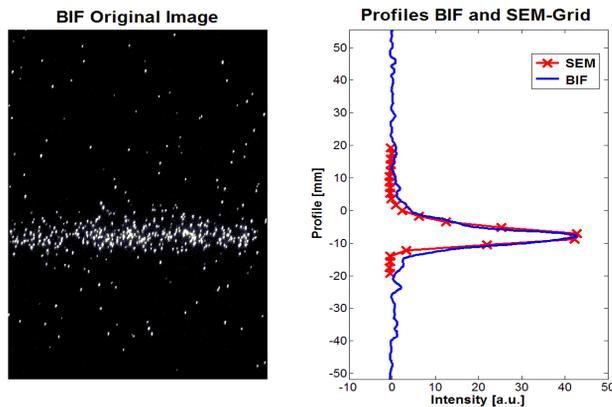
Figure 5: Single shot BIF image and profiles of BIF and SEM grid measurement, UNILAC section UA4 at 11.4 MeV/u, U 39+, 4·10<sup>10</sup> ppp and 5·10<sup>-6</sup> mbar N<sub>2</sub>.
