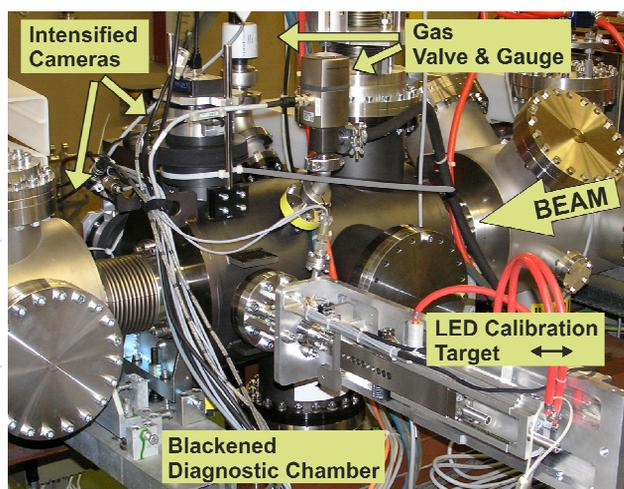
Figure 2: BIF installation at GSI UNILAC.
