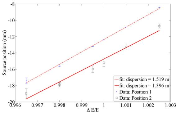
Figure 2: Example dispersion measurement.
