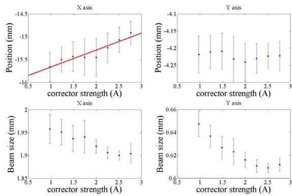
Figure 3: Position and size changes with horizontal corrector magnet strength changes.
