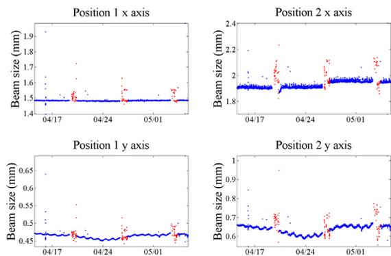
Figure 5: Beam size on both axes at the two SLMs over several user runs.
