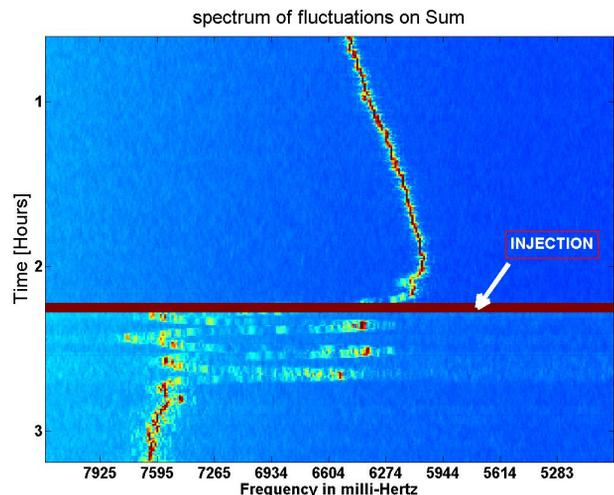
Figure 6: 3hrs monitoring at the moment of Injection of the exact frequency of the 6Hz line in the Sum spectrum.
