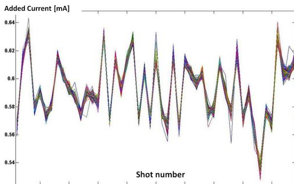
Figure 4: The ‘normalized-subtracted’ Sum signals of all BPM units in 224 curves over 50 injection shots. The average rms deviation between the 224 units is 0.35%.
