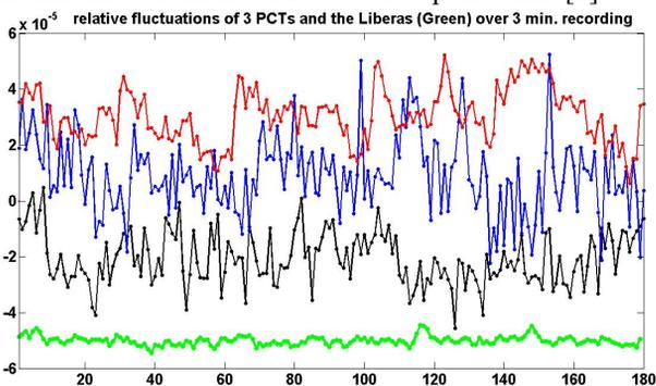
Figure 1: Comparative stability of current measurements between the 3 PCTs and the BPM-Liberas (in green).
