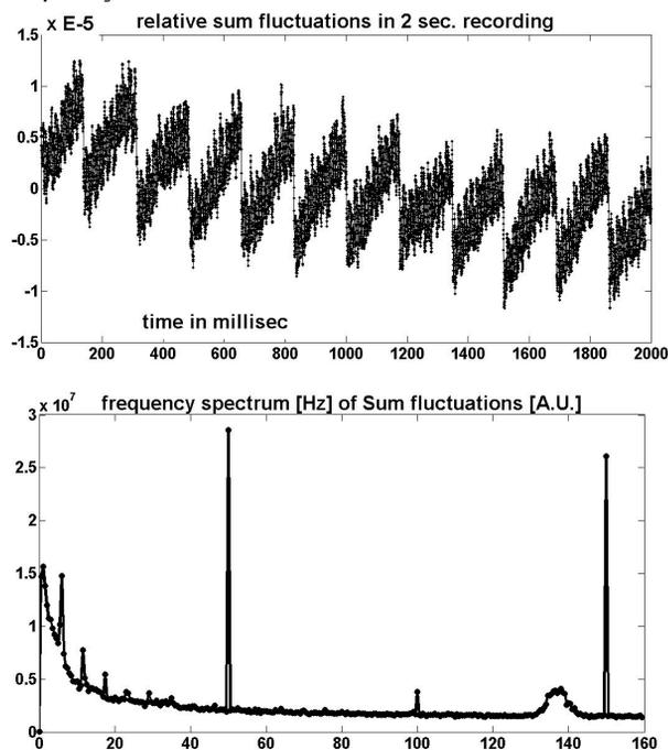
Figure 5a & 5b: Relative fluctuations of the Sum signal in a 2sec recording and its frequency spectrum.
