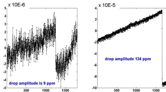
Figure 3: Examples (180sec at 10Hz) of instant-partial-beamdrops of only 9ppm (<2uA) and 134ppm. The normal beam lifetime slope is redressed in these curves.
