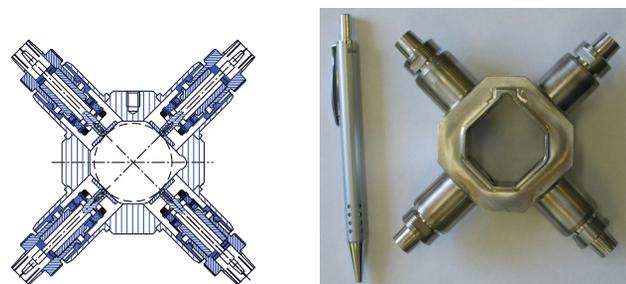
Figure 1: The beam position monitor for VEPP-2000 ring.
