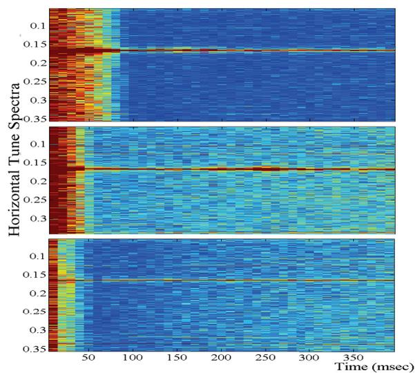
Figure 5: Horizontal tune measurements at injection energy of 11.4 MeV/u. At number of injected particles  $2.5 \cdot 10^{10}$  (Top),  $1 \cdot 10^{10}$  (Middle),  $2 \cdot 10^9$  (Bottom).
