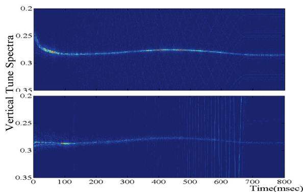
Figure 6: Vertical tune measurements at accelerating ramp from 11.4 - 600 MeV/u. At number of injected particles  $2 \cdot 10^{10}$  (Top),  $1 \cdot 10^{10}$  (Bottom).
