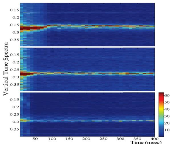
Figure 4: Vertical tune measurements at injection energy of 11.4 MeV/u. At number of injected particles  $2.5 \cdot 10^{10}$  (Top),  $1 \cdot 10^{10}$  (Middle),  $2 \cdot 10^9$  (Bottom).
