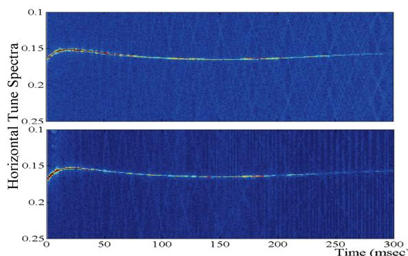
Figure 7: Horizontal tune measurements at accelerating ramp from 11.4 - 600 MeV/u. At number of injected particles  $2 \cdot 10^{10}$  (Top),  $1 \cdot 10^{10}$  (Bottom).
