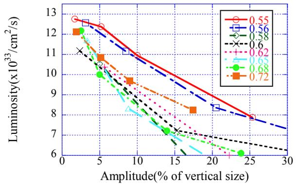
Figure 7: Luminosity degradation by the externally applied sinusoidal noise by the beam-beam simulation. The results are scaled to fit the experimental data.
