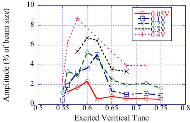
Figure 4: Beam response with the excited tune.
