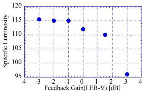
Figure 1: Luminosity reduction with the KEKB-LER vertical feedback gain.
