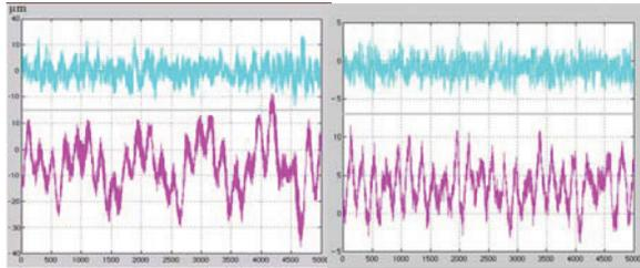
Figure 3: BPM signals with orbit correction ON (blue) and OFF (purple), H scale 50ms/div, V scale  $10\mu m/div$  (left plot) and  $5\mu m/div$  (right plots).
