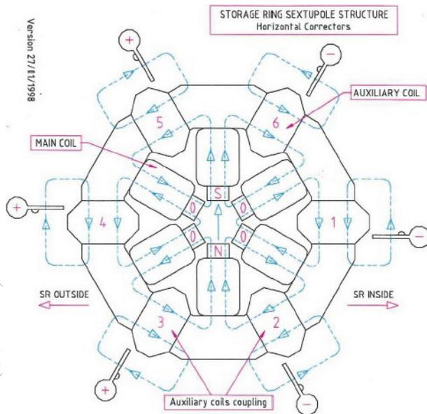
Figure 1: Layout of the auxiliary correctors in a sextupole.
