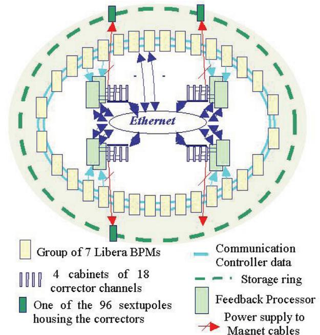
Figure 2: Layout of the future orbit correction system.
