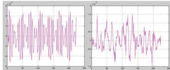
Figure 5: Horizontal (left plot) and vertical (right plot) response of the beam orbit to a horizontal kick of 150rad.
