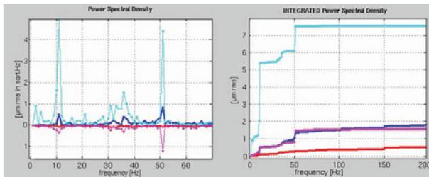
Figure 4: Power spectral density (left) and integrated power spectral density (right) averaged over the BPMs of the 2 corrected cells with and without orbit correction. Light blue, dark blue: H signals, purple, red: V signals
