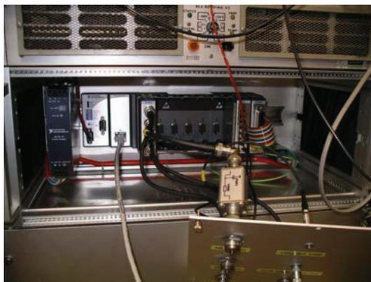
Figure 2: Photo of the opened system. The 8-slot CRIO system is visible as well as the ADC and DIO modules.
