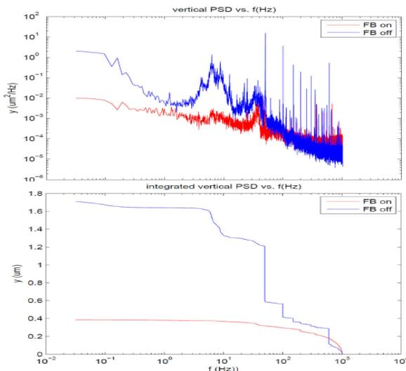
Figure 5: On top the vertical PSD, and below the SQRT of its integral, taken when FOFB is off and on.
