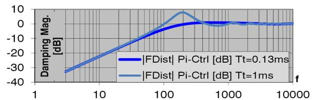
Figure 3: Analytic closed loop response, calculated for two different reaction times due to signal propagation.
