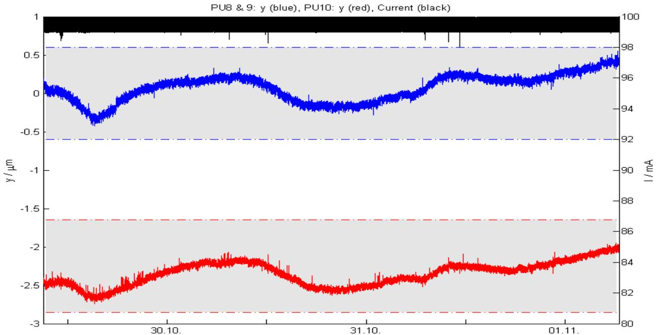
Figure 4: Vertical Long Term Stability at different undulator positions. 2010-10-29 to 2010-11-01.
