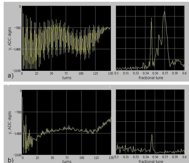
Figure 3: Beam injection: (a) 11 mA electron bunch with feedback off, (b) 11 mA electron bunch with feedback on.
