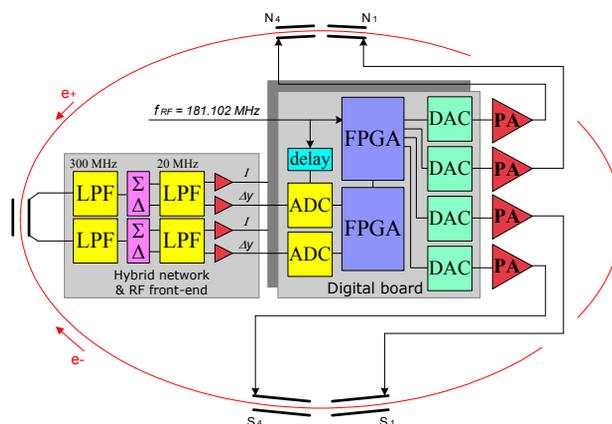
Figure 1: Block diagram of the VEPP-4M transverse digital bunch-by-bunch feedback system.
