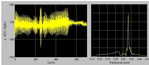
Figure 4: Beam oscillation excited by the feedback system for tune measurement.
