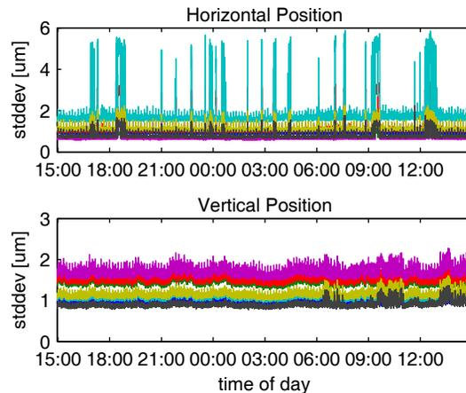
Figure 1: Standard deviation of EBPM position readings over a 24 h period. Colours represent 7 EBPMs in one cell.
