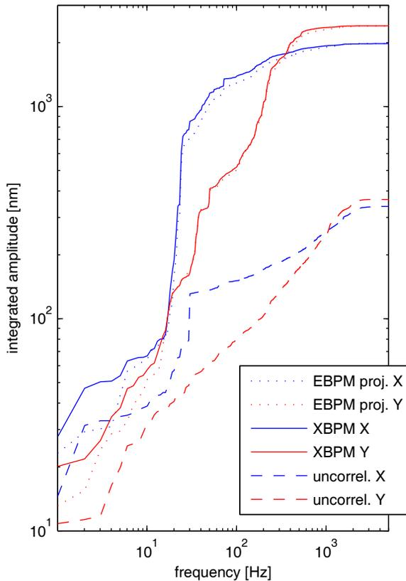
Figure 3: Integrated motion amplitudes of projected EBPM and XBPM positions (at the location of the XBPM), and uncorrelated components.
