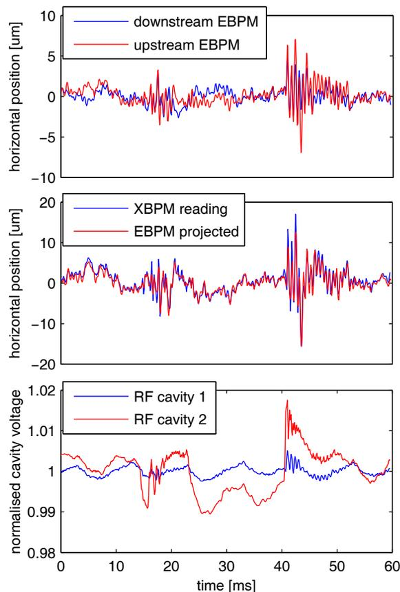
Figure 2: EBPM and XBPM position readings together with records of the RF cavity voltages with step changes.
