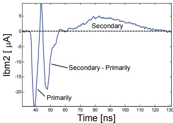
Figure 4: Dynamic of BM2 current at 5V potential of drift space ( $U_{bm1}=U_{drift}=U_{bm2}=5V$ ).
