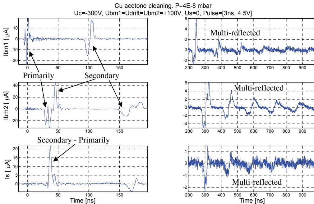
Figure 2: Typical current signals recorded from BM1, BM2 and “Sample”.
