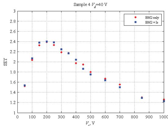
Figure 3: SEY of copper sample at residual gas pressure  $4 \cdot 10^{-8}$  mbar.
