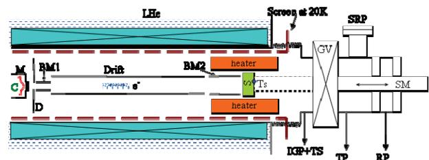
Figure 1: Experimental set-up. “SC” – superconducting coil, “C” – thermo-cathode, “M” – modulator, “D” – diaphragm, “BM1, BM2” – beam monitor (coaxial cylinders), “LHe” – liquid helium, “S” – sample, “Ts” – thermo sensor, “GV” – all metal gate valve, “IGP+TS” – ion getter pump + titanium sublimation pump, “TP” – turbo-molecular pump, “RP” – rough pump, “SRP” – sample replacement port, “SM” – sample manipulator.
